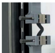
Angle tear strength
