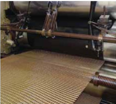
Polysur® Ferro SW-RE elevator belt during production
