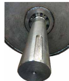
Shaft showing with 1 step juvination and with keyway
