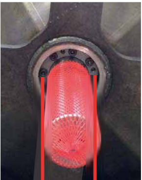
Bar pulley with internal double cone showing
