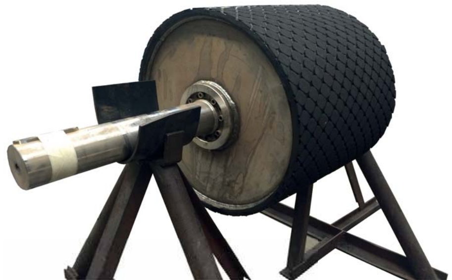
Detail of finished seams on rubber pulley lagging with paste
