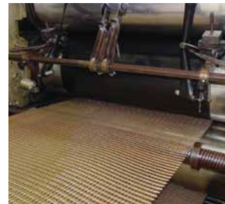
Polysur® Ferro SW-RE carcass during production
