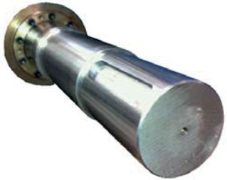
Shaft showing with 2 step rejuvenation and with keyway
