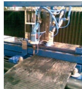
CNC drill unit for drilling elevator bucket bolt holes and belt fastener bolt holes in Polysur® FERRO steel cord reinforced elevator belt
