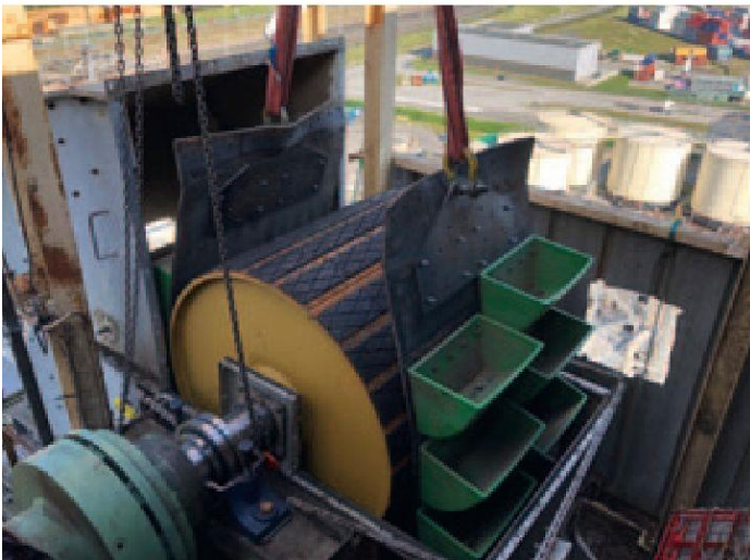
Fig. 4 The drive pulley is mounted in the head of the elevator
