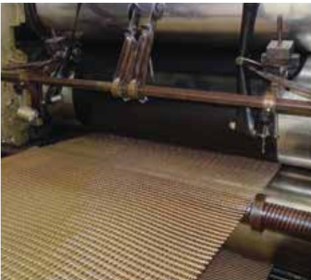
Polysur® Ferro SW-RE elevator belt during production
