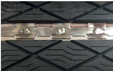
Close up of the Slide-Lag pulley lagging welded on the surface of the drive pulley
