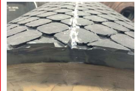
Detail of finished seams on rubber pulley lagging with paste
