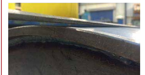
Close up of crowing on drive pulley surface
