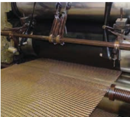
Polysur® Ferro SW-RE carcass during production
