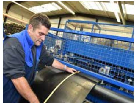
Polysur® EP textile reinforced rubber elevator belt provided with CNC punched elevator bucket bolt holes. Two rows of elevator buckets situated in staggered pattern on the elevator belt
