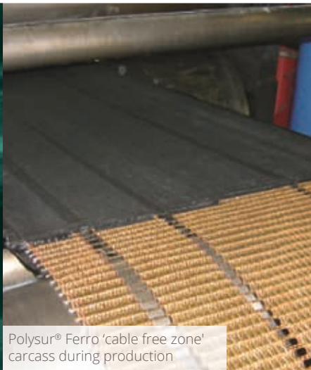
Polysur® Ferro SW-R/RE 'cable free zone' carcass
