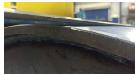
Close up of crowning on drive pulley surface
