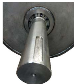
Shaft showing with 1 step juvenation and with keyway
