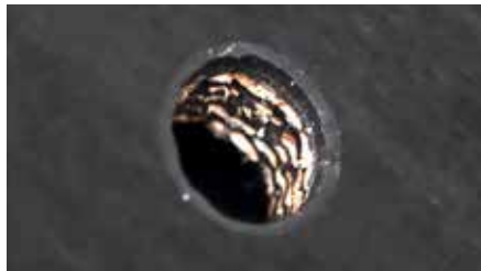
CNC punched elevator bolt hole in Polysur® EP textile reinforced rubber elevator belt
