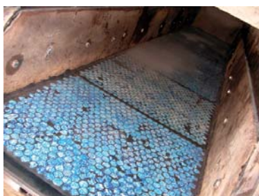
REDI-LINER™ type KT installed in gliding chute for handling recycled asphalt
