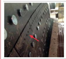
Replaceable oil and grease-resistant wear rubber fitted on the aluminium wedge part of the fastener by two Allen bolts.
