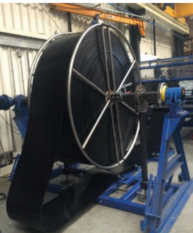
Decoiling the Polysur® Ferro belt in the CNC bolt hole drilling machine
