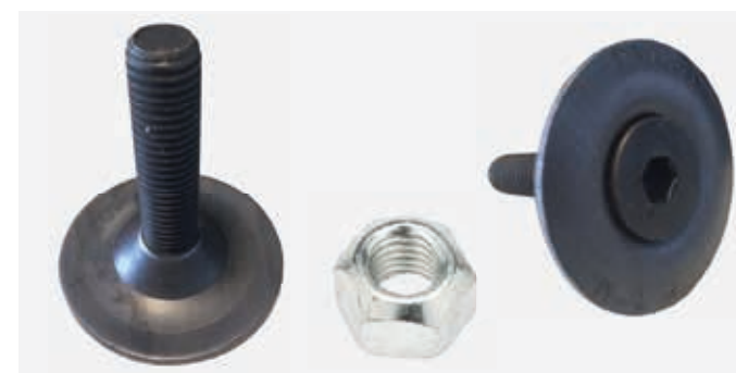
PTM style M12, 10.9 grade elevator bolt with Ø 50 mm bolthead and allen key. Complete with heat resistant M12 DIN 980V lock nut
