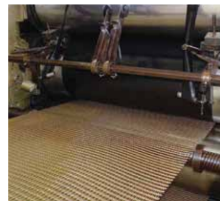
Polysur® Ferro SW-RE carcass during production
