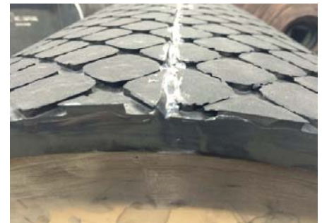
Detail of finished seams on rubber pulley lagging with paste
