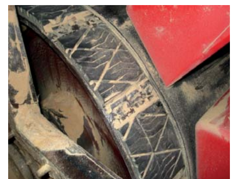
Close up of the Slide-Lag pulley lagging welded on the surface of the drive pulley
